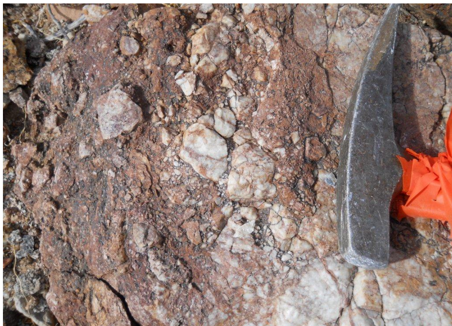
Photo 8: Brecciation in a 20 to 50 cm thick zone of multiphase faulting and quartz veining that cuts granodiorite at UTM 341325E-3393854N. Faint green staining may be an arsenic oxide. Sample GRM-06 assayed 1.04 g/t Au and 23.9 g/t Ag (Table 5).
