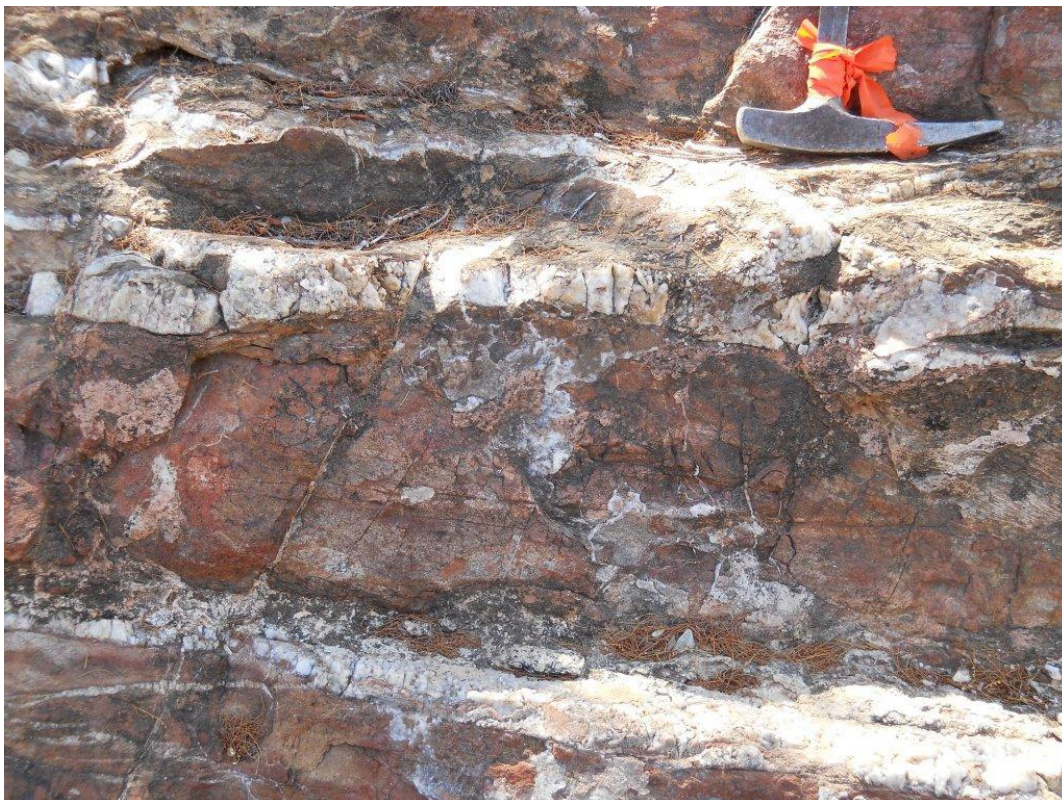
Photo 7: A series of parallel quartz veins, up to 2.5 cm thick, confined to a 40 cm wide fracture zone at UTM 341430E-3393738N. The veins, which cut a weathered ?andesite dike, strike SE and dip 43 degrees SW. Sample GRM-04 from the veins assayed 0.53 g/t Au (Table 5).
