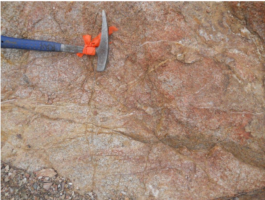
Photo 6: A stockwork of thin, NNE trending, sub-vertical quartz stringers that cut strongly weathered granodiorite at UTM 341086E-3393815N. Sample GRM-02 from the veinlets assayed 0.08 g/t Au (Table 5).
