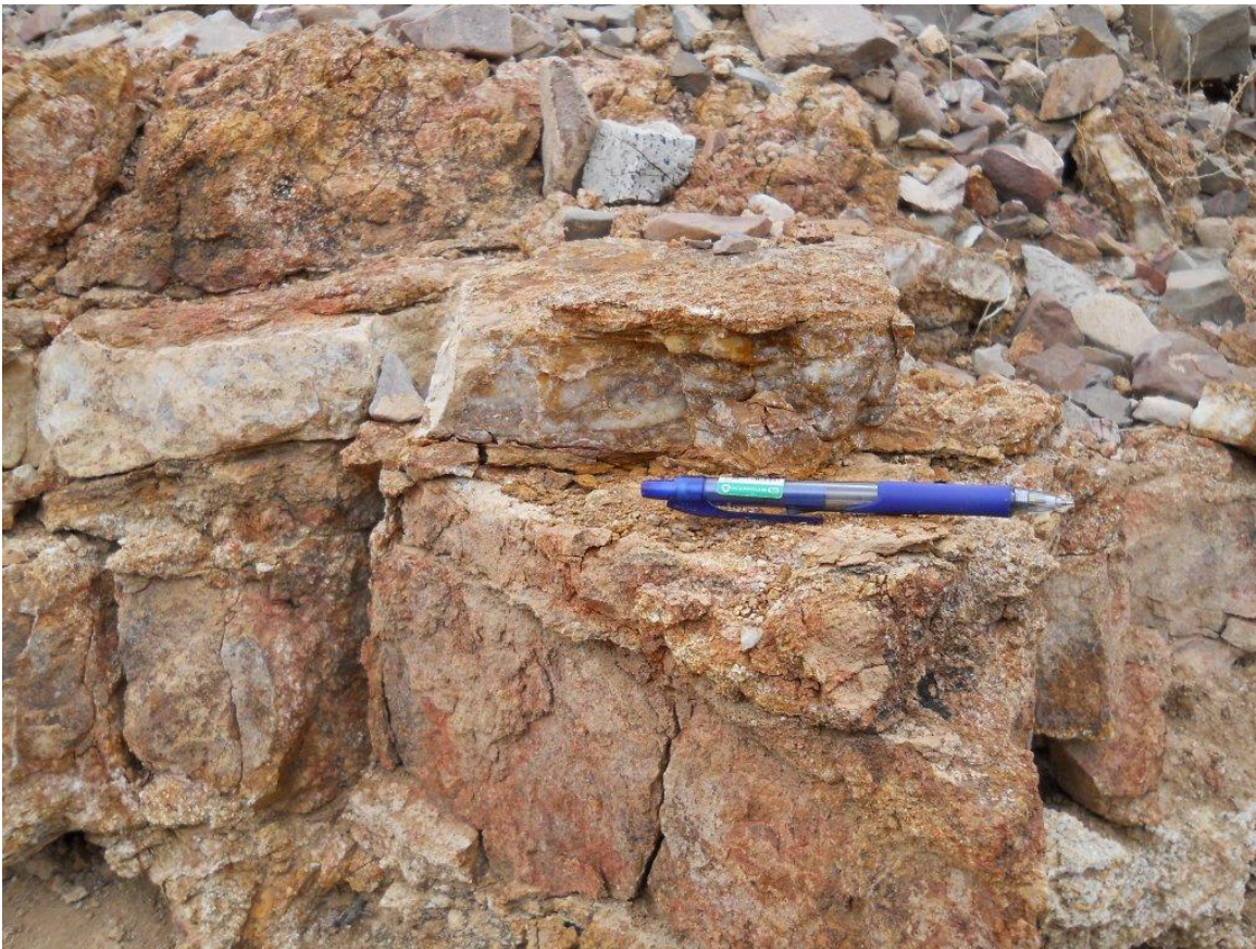
Photo 4: A flat-lying, 4 cm thick quartz vein cutting strongly weathered granodiorite at UTM 341086E-3393815N. Sample GRM-01 from the vein assayed 0.49 g/t Au (Table 5).
